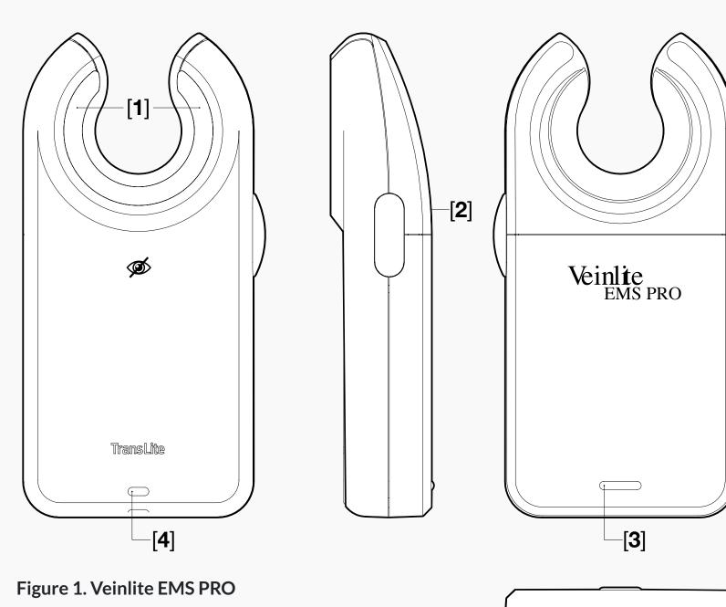
[1] Clear Window [2] On/Off Mode Toggle Switch Button with Low Battery
